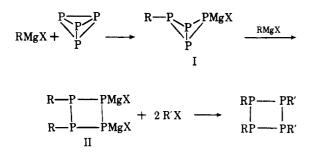
It is likely, however, that the process is complicated by reaction of intermediates I and II with unchanged  $P_4$ to give more complex phosphides, which in turn are broken down.
